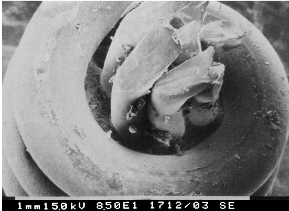
Fig 10. A scanning electron micrograph of a cross-section of a biopsy forceps after cleaning demonstrating residual organic soil. This image demonstrates the difficulty of cleaning all of the internal surfaces of these complex devices. Scanning micrographs by Walter Bond.
